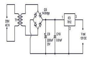
Available power source is an AC voltage arrives at 230V. Since our electronic circuit require only very minimal voltage and current. We use step down power transformer. Step down transformer is designed in away such a way that the input is 230V and the output is 12V.
